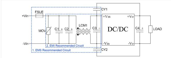
Note: Part 1 in the figure is for EMS testing, and part 2 in the figure is for EMI filtering, which can be adjusted according to the situation.
